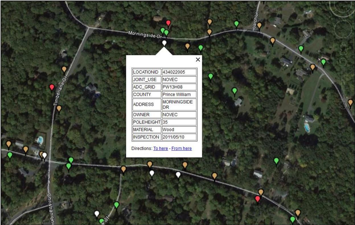
**Figure 21: 3PA Tree-Trimming Circuit Map**
